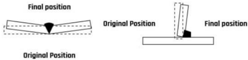
Figure 4. Butt-joint and T-joint Source:( https://technoweld.com.au/2019/07/30/basics-of-distortion-in-welding/ )
